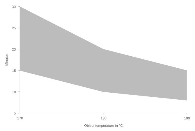
**T** Object **t** min **t** max 170 °C 15 minutes 30 minutes 180 °C 10 minutes 20 minutes 190 °C 8 minutes 15 minutes
