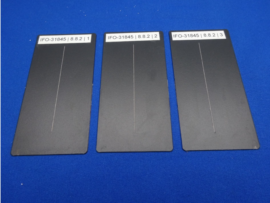
Figure 13 – Samples after Salt Spray Resistance test (see Ch. 2.8.2: Test acc. to AAMA 2604-20, Ch. 8.8.2)
