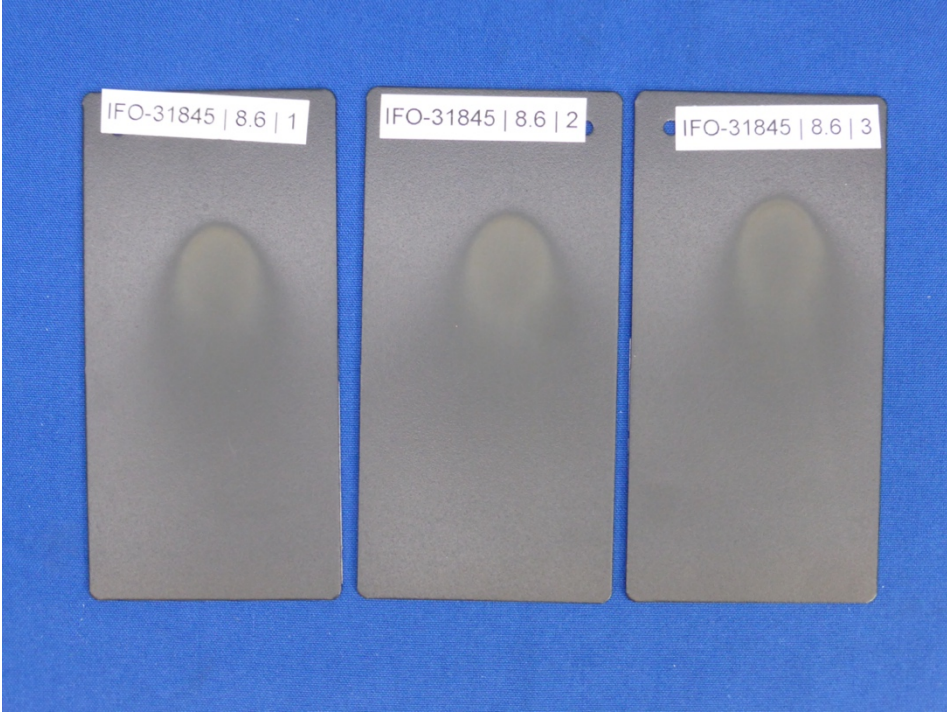
Figure 6 – Samples after Abrasion Resistance test (see Ch. 2.6: Test acc. to AAMA 2604-20, Ch. 8.6)
