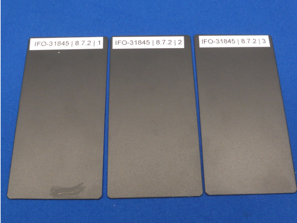
Figure 8 – Samples after Mortar Resistance test (see Ch. 2.7.2: Test acc. to AAMA 2604-20, Ch. 8.7.2)
