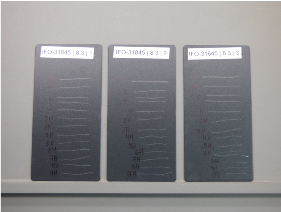
Figure 3 – Samples after Dry Film Hardness test (see Ch. 2.3: Test acc. to AAMA 2604-20, Ch. 8.3)
