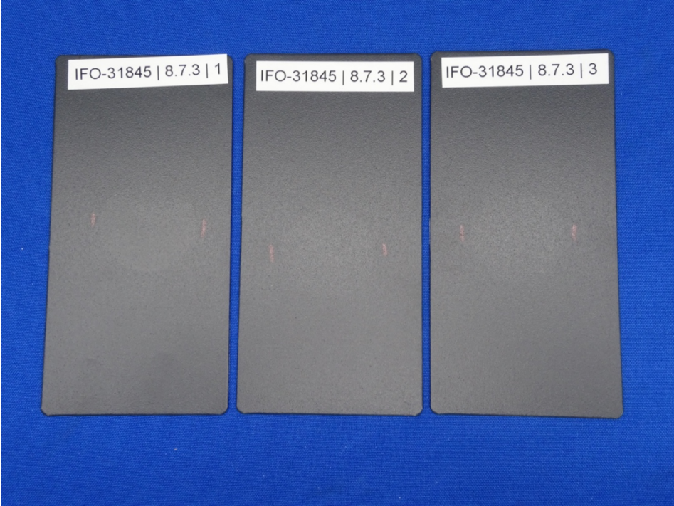
Figure 9 – Samples after Nitric Acid Resistance test (see Ch. 2.7. 3: Test acc. to AAMA 2604-20, Ch. 8.7.3)
